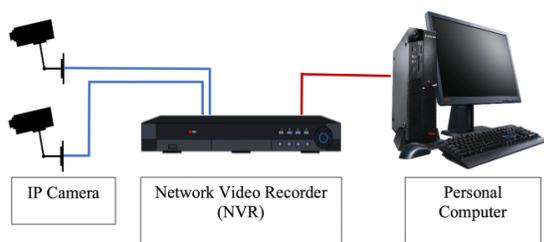
**Fig. 1** Network diagram of molting detection system including IP camera, NVR, and personal computer. All components were connected by local-area network (LAN) cable.
