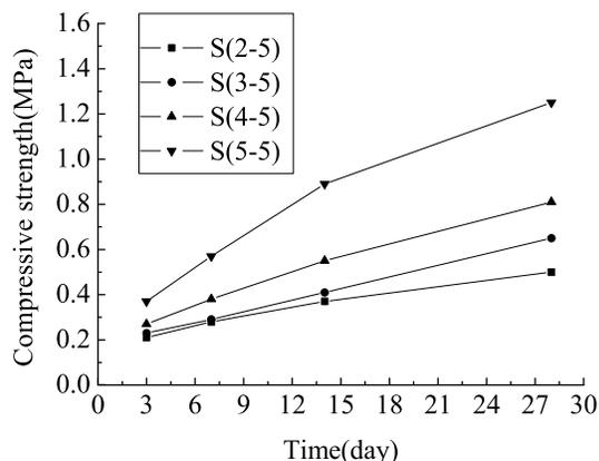
**Fig. 1** Strength developments of the samples with mass ratio of SBSM/sewage sludge of 5%.
