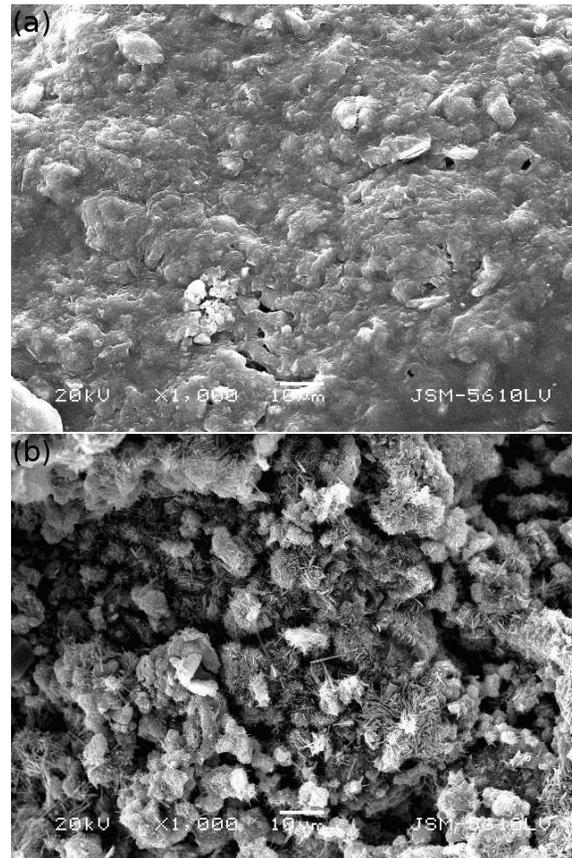
**Fig. 4** Scanning electron microscopy images of the samples: (a) unsoldified sewage sludge and (b) sample S(5-10) cured under laboratory conditions for 28 days.
