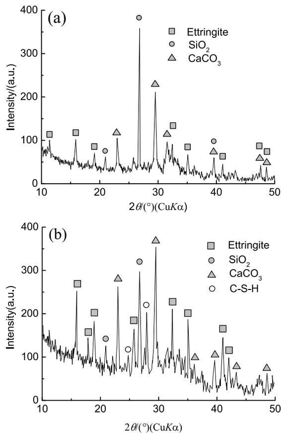
**Fig. 3** X-ray diffractograms of the solidified pastes (a) S(3-10) and (b) S(5-10) cured under laboratory conditions for 28 days.
