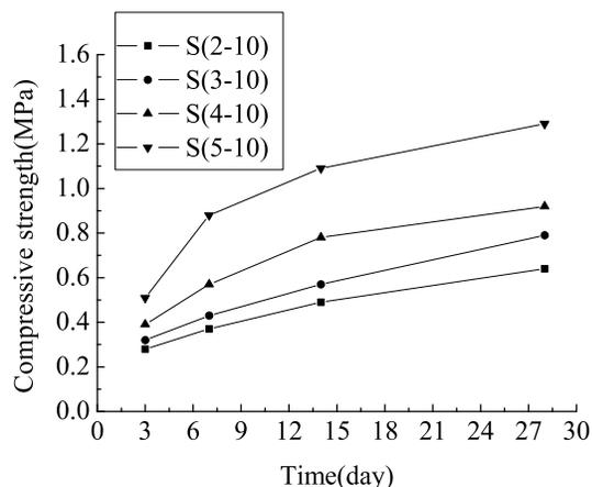
**Fig. 2** Strength developments of the samples with mass ratio of SBSM/sewage sludge of 10%.
